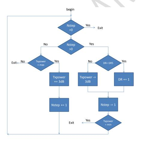
Note: In the case where Nstep is negative and TXPower is already at its maximum the algorithm does not try to lower the data rate, because the end-device's implements automatic data rate decay. The algorithm can only actively increase the data rate. Trying to lower the data rate leads to constantly oscillating values.
