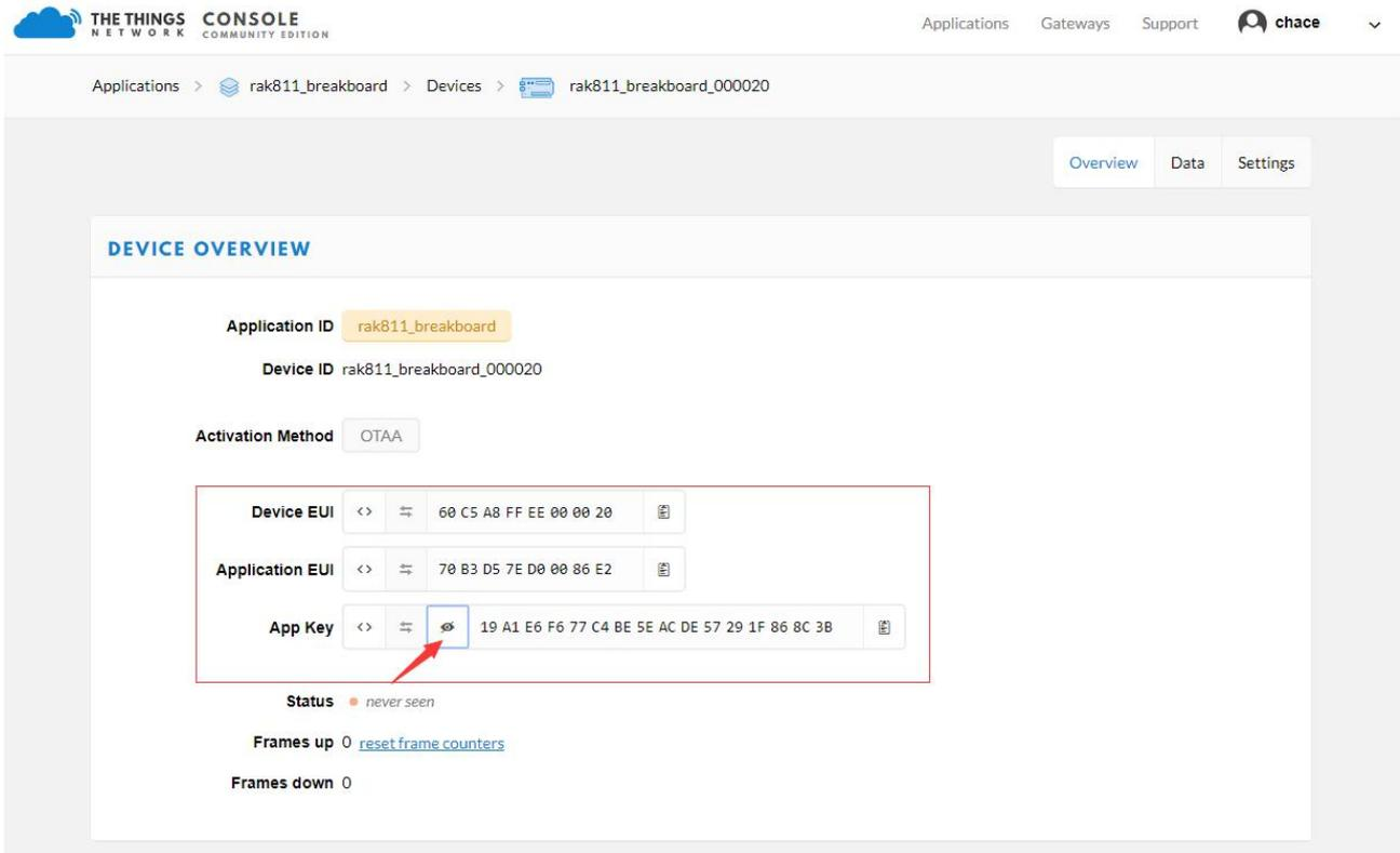
After obtaining three parameters of Devices EUI, App EUI and App key, open the ClassA project of RAK811 BreakBoard open source code and modify these three parameters. Then compile the download process.
