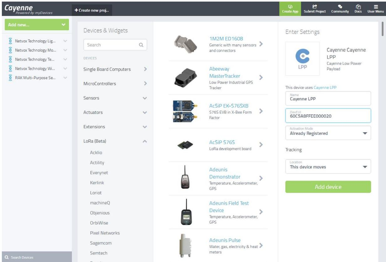
Finally click Add Device, the device is added successfully. Next you need to set the parameters of the TTN interface.
