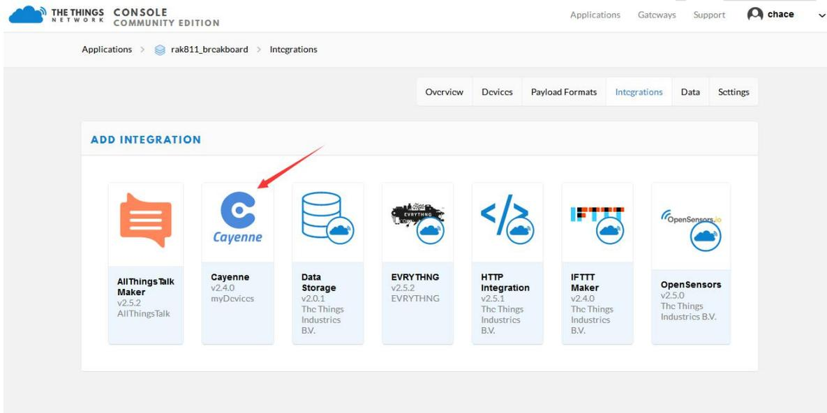
After entering the setting interface, the Process ID can fill in any name, eg: lora\_button. The Access Key is set default key..then click Add Integrations. So Cayenne is added.
