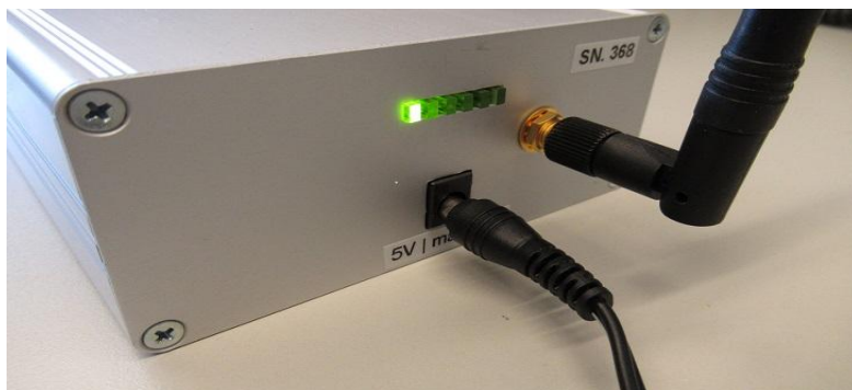
Figure 4 Connection RF antenna and power supply
