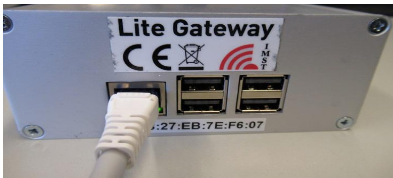
Figure 3 Connection Ethernet cable
